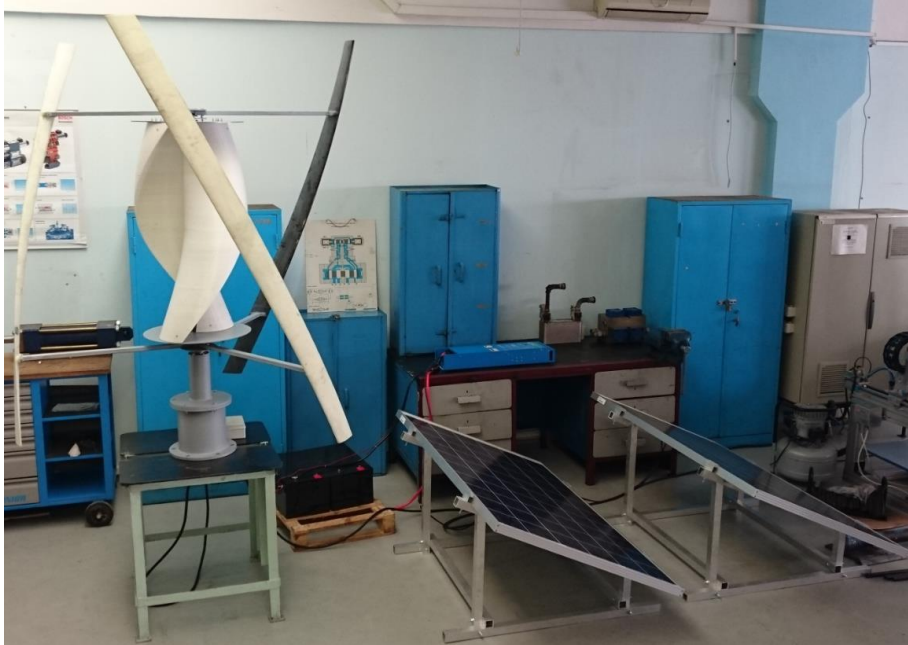
Fig. 6. Model experimental de sistem combinat electric cu rotor Savonius
